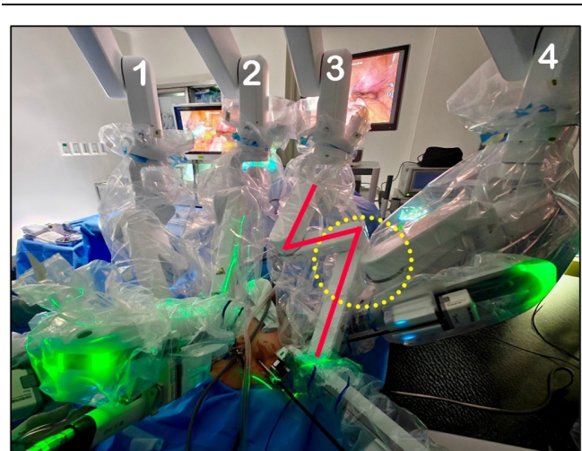
Figure 3. Maximizing the lateral tilt of arm 3. The figure shows how arm 3 (red line) achieves maximum lateral tilt by sliding medially to arm 4 (yellow dotted circle).
